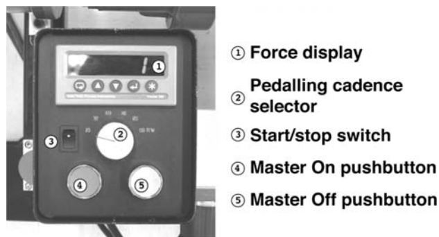
Fig. 3 Control panel of the calibration rig
