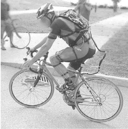
Fig. 4. Cyclist and bicycle equipped with the dynamometric hubset and data acquisition system attached to a modified backpack
