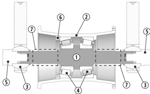
Fig. 2. Sectional view of the front hub with component identification: 1-axle, 2-body, 3-spherical bearings (rod ends), 4-wheel bearings, 5-axle bolts, 6-lock ring, 7-strain gauge instrumented area of the axle
