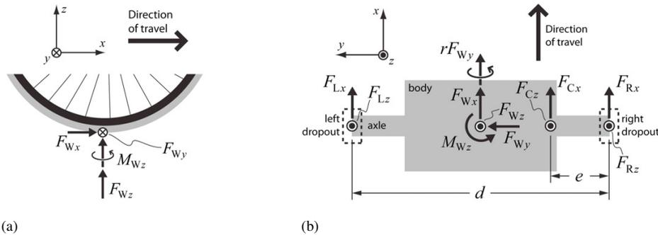
Fig. 3. (a) Ground contact reaction loads acting at the wheel and (b) Hub free-body diagram (Note 1: top view shown;  $F_{Cx}$  and  $F_{Cz}$  must be set to zero for the front hub; Note 2: The local coordinate system  $x$ - $y$ - $z$  is attached to the axle)
