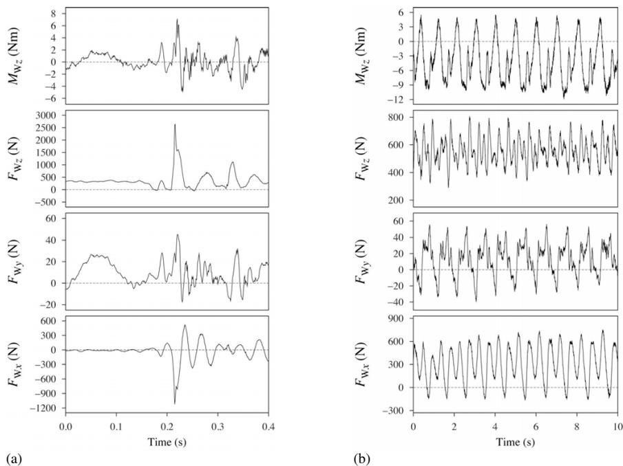
Fig. 5. Ground contact reaction loads measured (a) during road impact while coasting (front hub) and (b) when climbing out of the saddle (rear hub)
