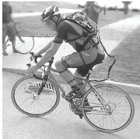
Fig. 4. Cyclist equipped with the data acquisition system attached to a modified backpack
