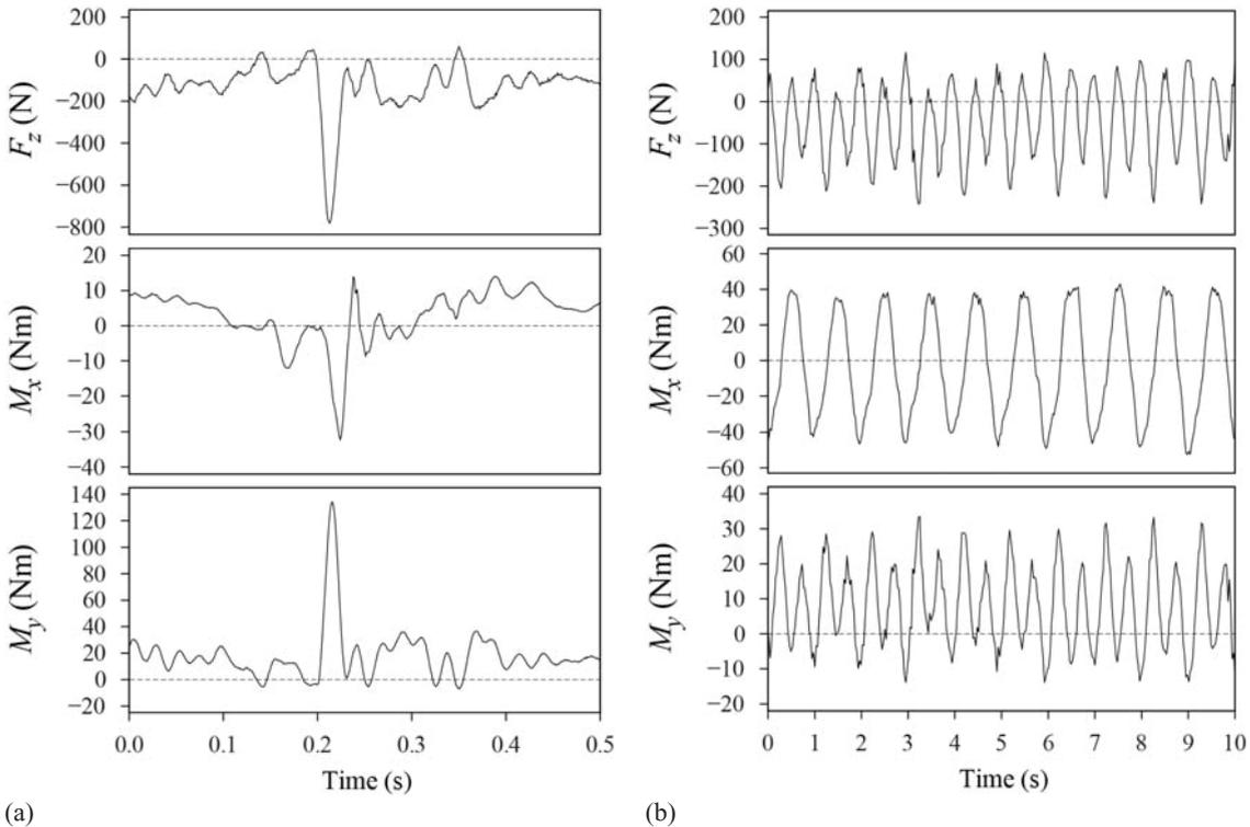
Fig. 5. Stem loads measured (a) during road impact while coasting and (b) when climbing a hill out of the saddle
