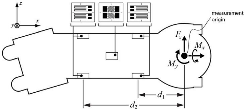
Fig. 2. Side view of the instrumented stem with measured loads, location of bridges #1 and #2, and strain gauge identification
