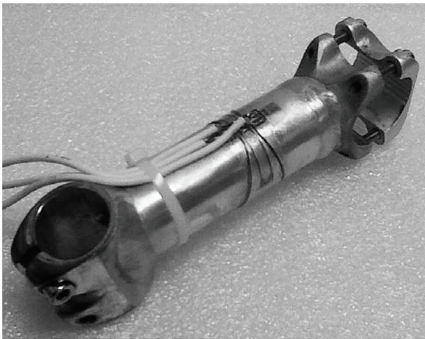
Fig. 3. Photograph of the instrumented stem
