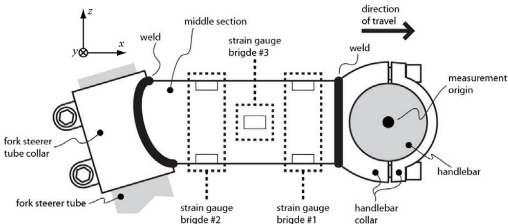
Fig. 1. Side view of the instrumented stem with strain gauges bridges and measurement origin identification
