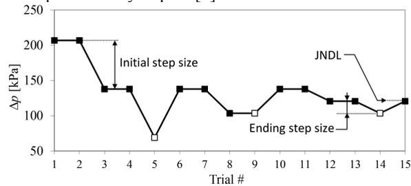
Fig. 2. Typical one-up two-down JNDL assessment procedure.
